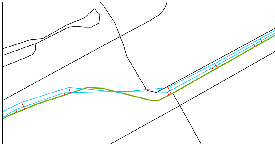
Figure 5. Two cycling traces (light blue) matched to the OSM base map roads (black) and the final road match result (green). The algorithm handles the matching of a single trajectory even when the trajectory is deviated to an adjacent road, or when the trajectory does not go through a junction.
